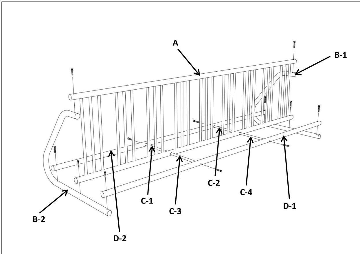
**Step 1:** According to diagram, attach two ends B-1 and B-2 to A.
