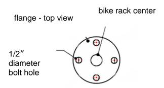
**Note:** Surface mounting hardware sold separately. Use 3/8" x 4" lag bolts. It is recommended that concrete cure 28 days prior to mounting.
