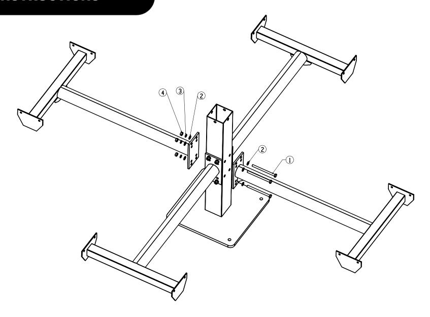
Attached the side frames to the pedestal frame using the specified hardware.
