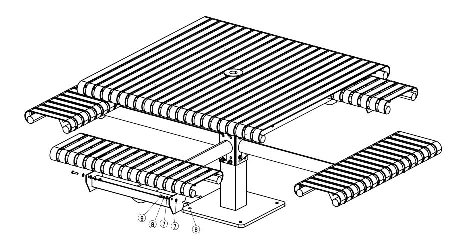
Attached the seat tops to the side frames using the specified hardware.
