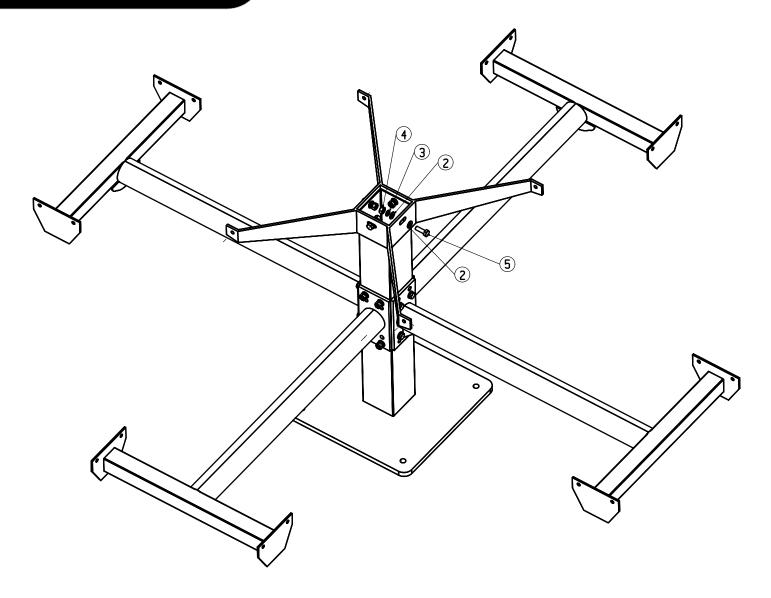
Attached table support bracket to the pedestal frame using the specified hardware.
