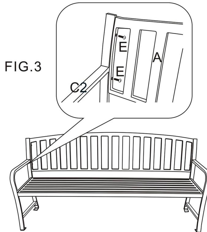
**Step # 4:** Adjust the bench to a level position and tighten all the Bolts with Allen Wrench (F) (Provided).
