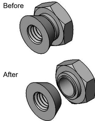
Hex part of nut will break off when tightened to 185in-lbs.
